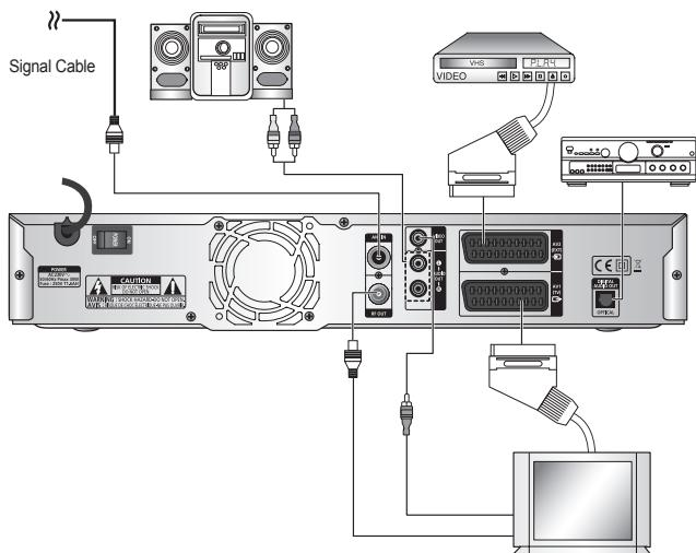
If degraded picture quality is observed while viewing copy-protected VOD (Video-on-Demand) movies, connect the set-top box directly to the TV set. Do not connect through a VCR.
