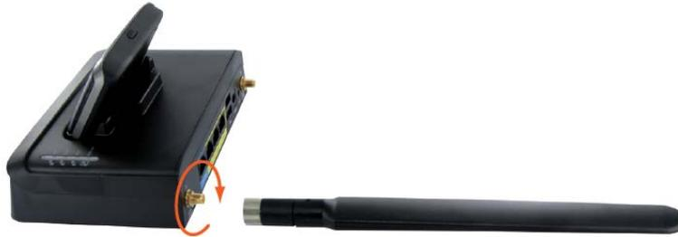
2. Turn the metal part to screw in the antenna until it tightens, then hold the metal part while turning the antenna to a vertical position.
