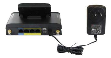
**4.** Follow the instructions provided with your AirCard mobile hotspot to connect to the Internet. Then dock the AirCard mobile hotspot into the AirCard Hub.
