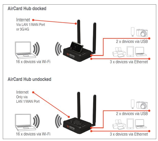
Figure 12: Power User Mode – AirCard Hub Docked/Undocked Scenarios
