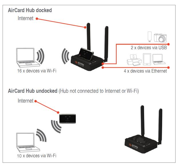
Figure 3: Easy Mode – AirCard Hub Docked/Undocked Scenarios
